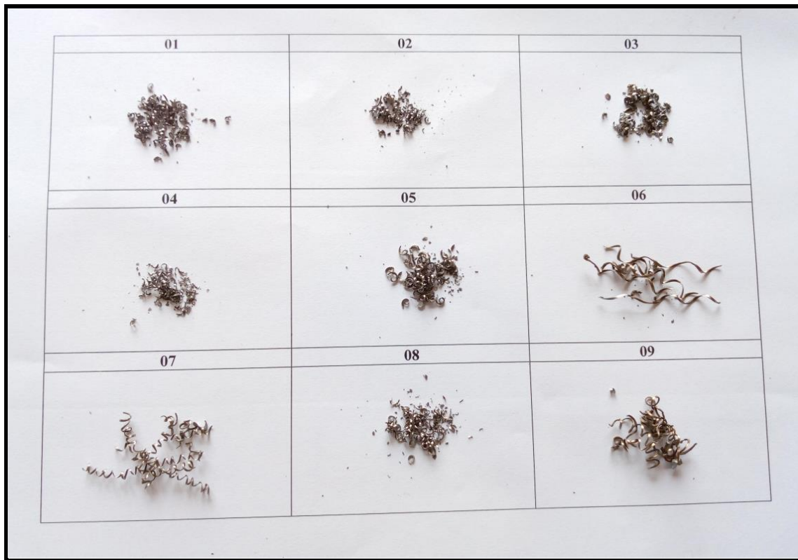
Fig 3: Forms of chip generated at varying machining conditions.
