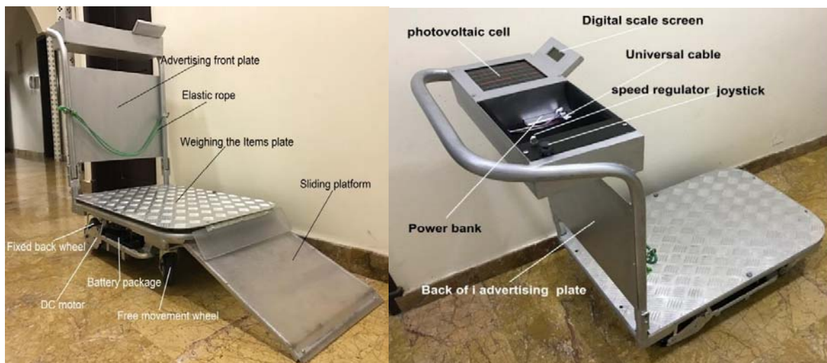
Figure 5 Two different views of the complete assembly of the trolley
