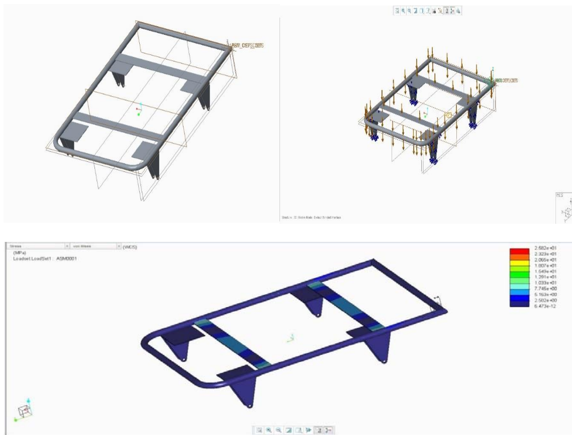
Figure 4 Stress analysis of the trolley structure using PTC Creo v3 software
