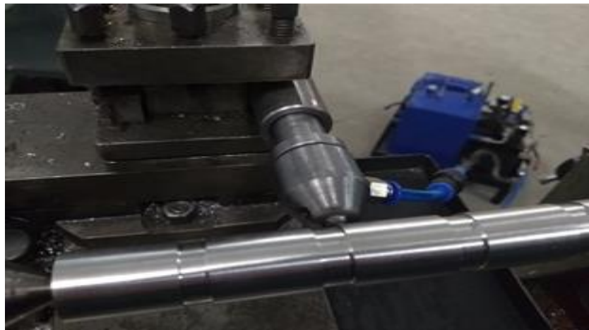
Figure 1. Burnishing process carried out on the specimen
