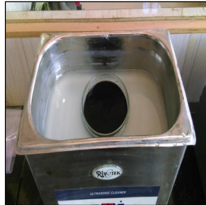
Figure 2. Carbon nano tube (CNT) kept in the Ultrasonicator
