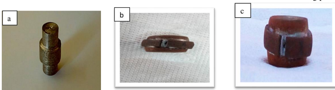
Figure 7 . Specimens (a) Before upsetting, (b) and (c) after upsetting
