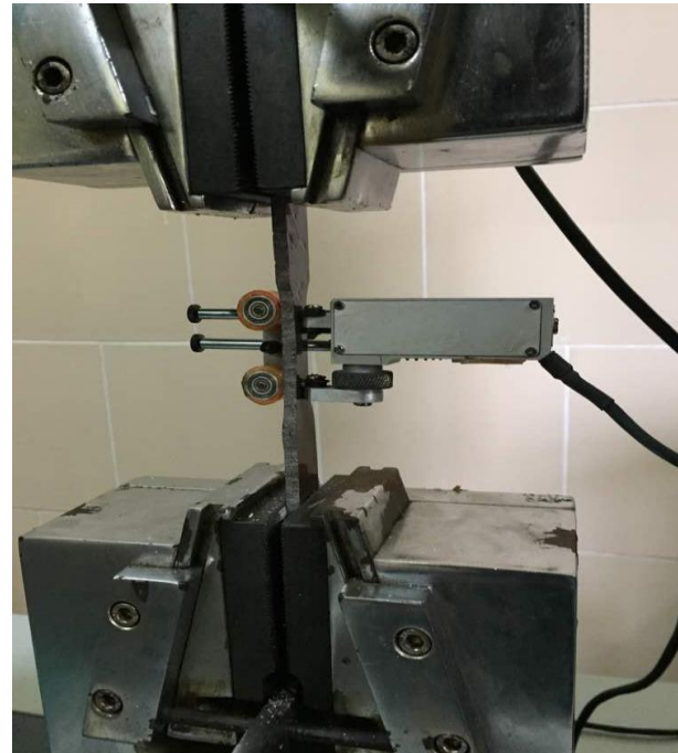
Figure 2 Universal Testing Machine - Tensile test
