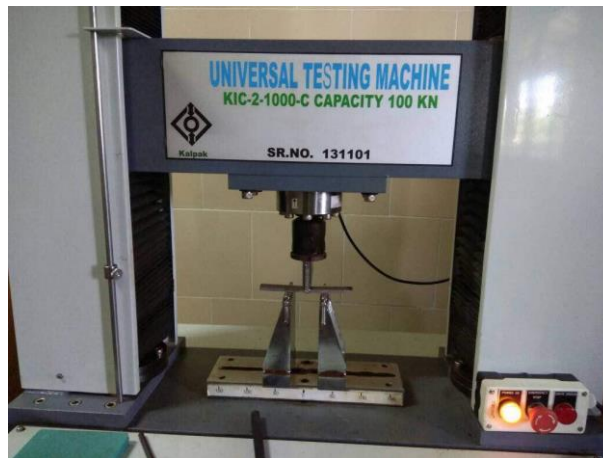
Figure 3 Universal Testing Machine - Bending test
