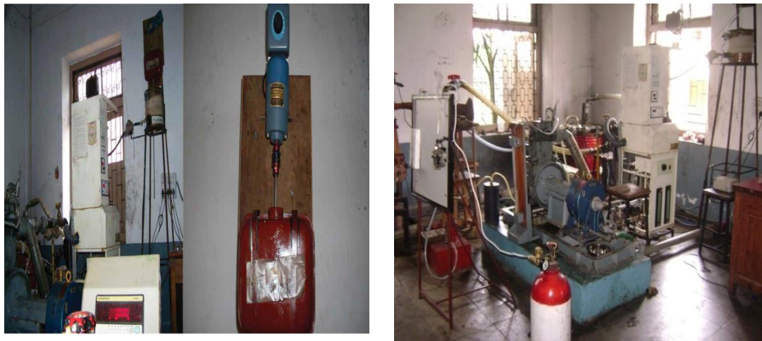
Figure 1. Engine test rig with ethanol mixing tank
