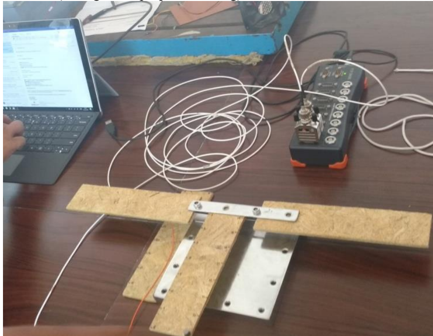
Figure 3.3 Dynamic Testing Setup.
