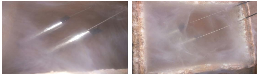
Figure 2.5. Specimens immersed in liquid nitrogen tank for 24 hrs and 48 hrs
