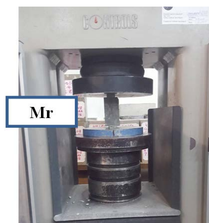
Figure 13. Effective compression test for sample Mr.
