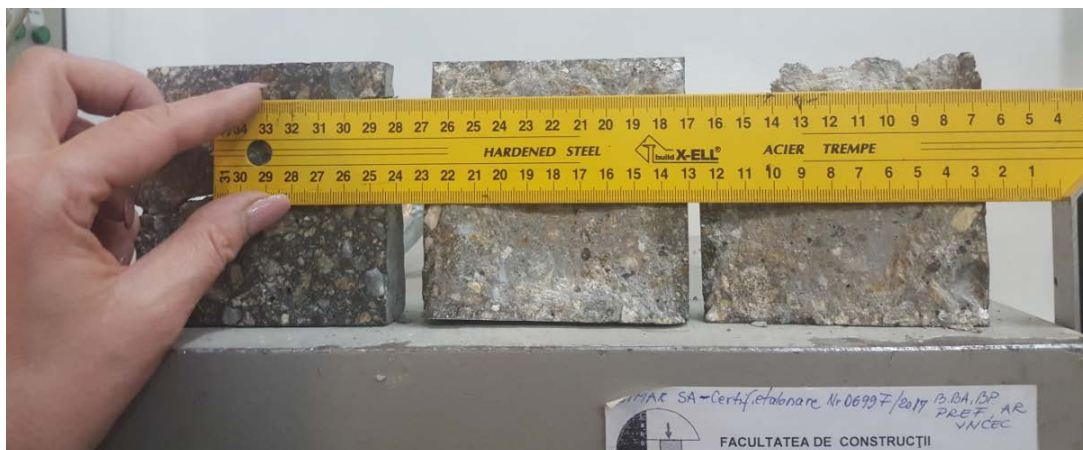
Figure 11. Water level penetration of control mix Mr.
