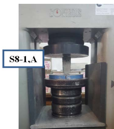
Figure 12. Effective compression test for sample S8-1,A.
