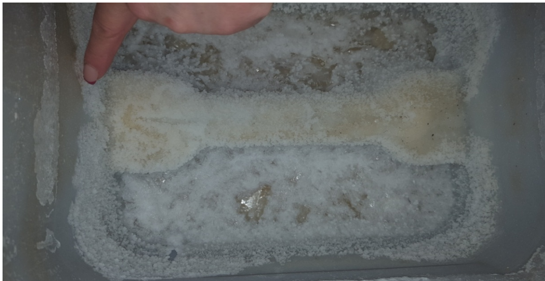
Figure 7. Salt deposits after the evaporation of concentrated saltwater from Oglinzi Baths.
