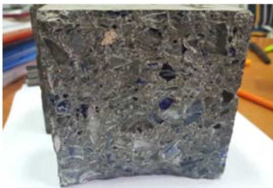
Figure 8. S8-1,A after immersion in saltwater.
