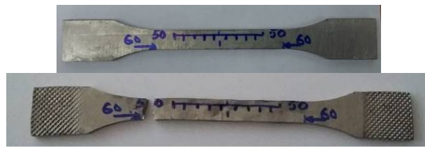
Figure 1. Continuous tensile test specimen, dimensions: 9.54x3.99 mm and L_c=105 mm, before and after fracture.
