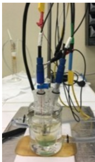
Figure 5. Electrochemical cell used in corrosion tests.
