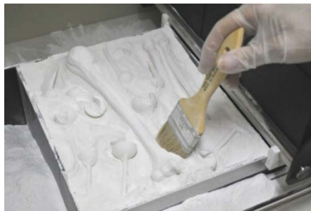
Figure 9. Extraction of prototypes from the powder tank.
