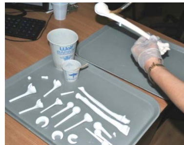
Figure 10. Infiltration with epoxy resin.
