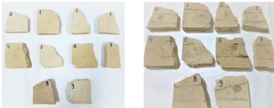
Figure 3. Calcareous porous sample: left – at 96h after chemical treatment (AT); right – testing hydrophobization efficiency after exposure period (178 days) in ambient urban air (ATE) and dried in 96h, in laboratory conditions.
