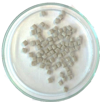
Figure 1. RPP waste used for the preparation of the lightweight concrete mixtures.
