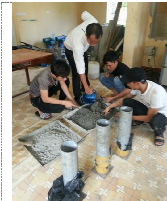
Figure 3. Manufacturing of CFST specimens.
