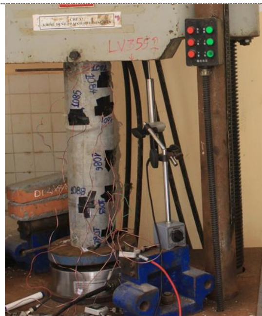
Figure 4. Test setup for CFST column.
