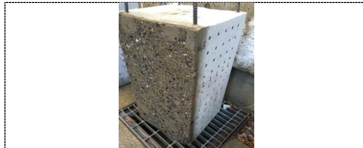
Figure 6. Concrete prism specimens with a deteriorated surface.
