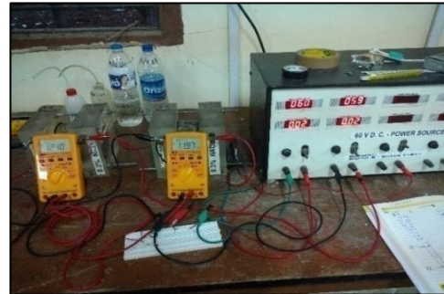
Figure 2. Typical laboratory test setup for RCPT.
