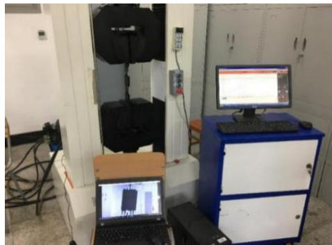
Figure 3. Universal testing machine pullout experiment platform.
