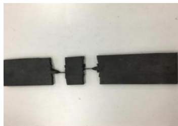
(b) Both sides of a single steel cord
