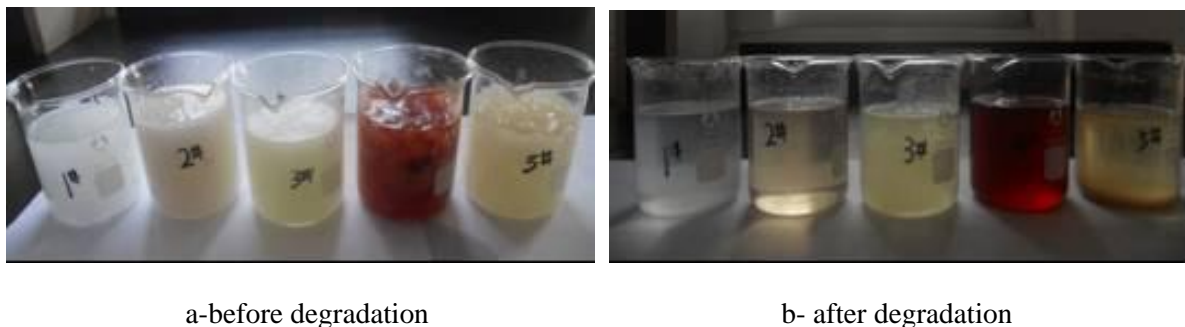
Figure 6. Fiber dispersion in different kinds of fluid and experimental photos after degradation.
