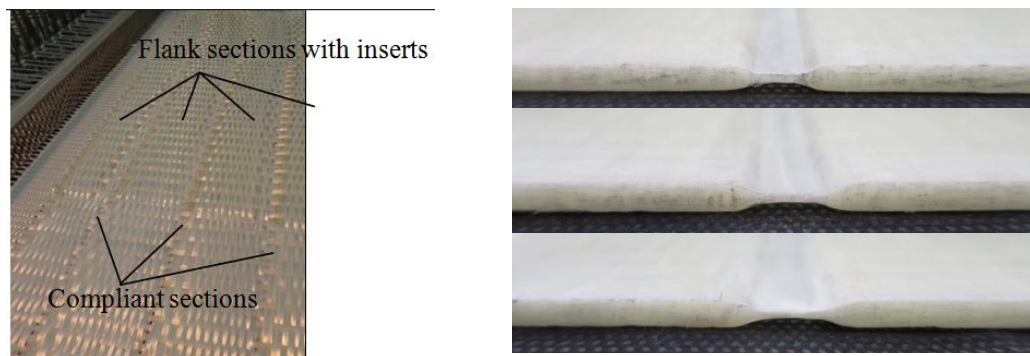
Figure 7. Weaving of compliant and flank sections of PACS using hybrid yarns and consolidated structures with different geometries of compliant section.
