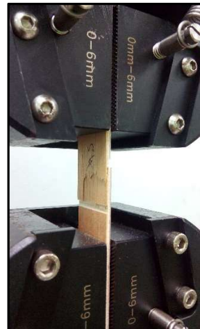
Figure 2. test specimen grip position
