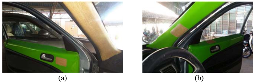
Figure 8. Composite parts consists of upper parts of door panel and pillar A (a) left side of car door (b) right side of car door.
