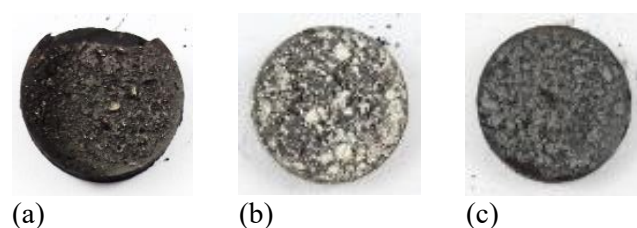
Figure 7. Double layer after sintering process: (a) NiO/Perovskite (b) CeO 2 /Perovskite (c) NiO-CeO 2 /Perovskite
