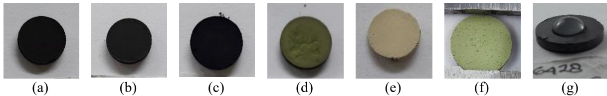
Figure 2. Single layer membrane of (a) LSCF 6428, (b) LSCF 7328, (c) LSM 73, (d) NiO, (e) CeO 2 , (f) NiO-CeO 2 and (g) example of drop water test result
