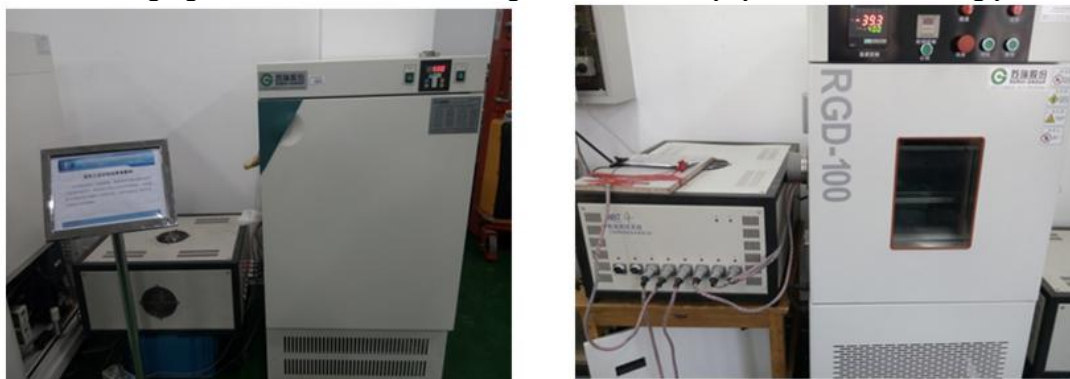
Figure 2. Battery float charging test platform
