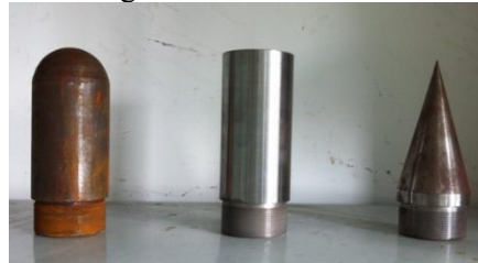
(a) Hemispherical rod electrode (b) Flat rod electrode (c) Conical rod electrode
