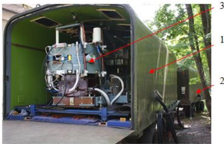
Figure 5. The photo of a single-beam three-frame mobile cyclic accelerator:
