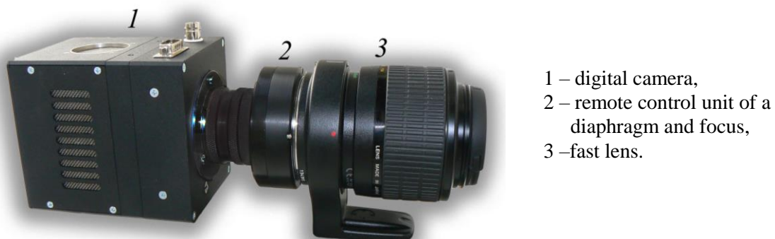
Figure 2. A channel of the multiframe recording system of the radiographic complex.
