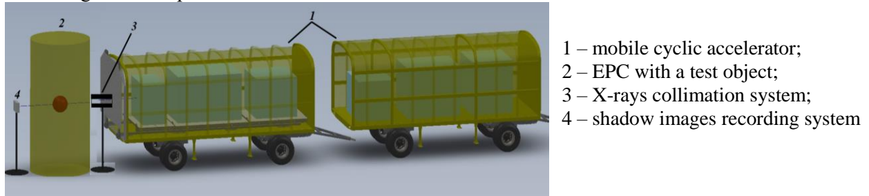
Figure 1. The experiment sketch with the usage of a single-beam three-frame mobile radiographic complex.
