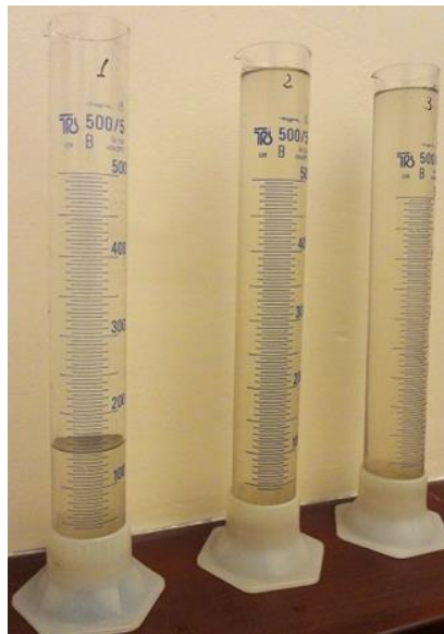
Figure 11. Experimental investigation of sedimentation characteristics of water samples
