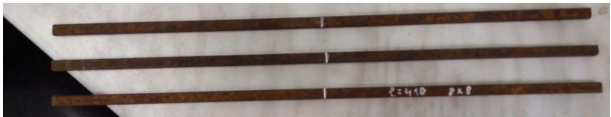
Figure 2 b. Tensile test specimens
