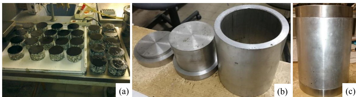
Figure 4. Finely polished base course surfaces with applied bitumen emulsion (a), opened compaction device (b) and closed compaction device (c)
