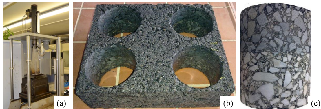
Figure 1. Roller sector compactor (a), two-layered asphalt slab (b) and specimen (c)
