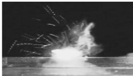
Figure 2. Photo. A fluid fountain formed by the radiation of an ultrasonic beam from the depth of the liquid to its surface (the radiation frequency is 1.5 MHz, the intensity is 15 W / cm 2 ).
