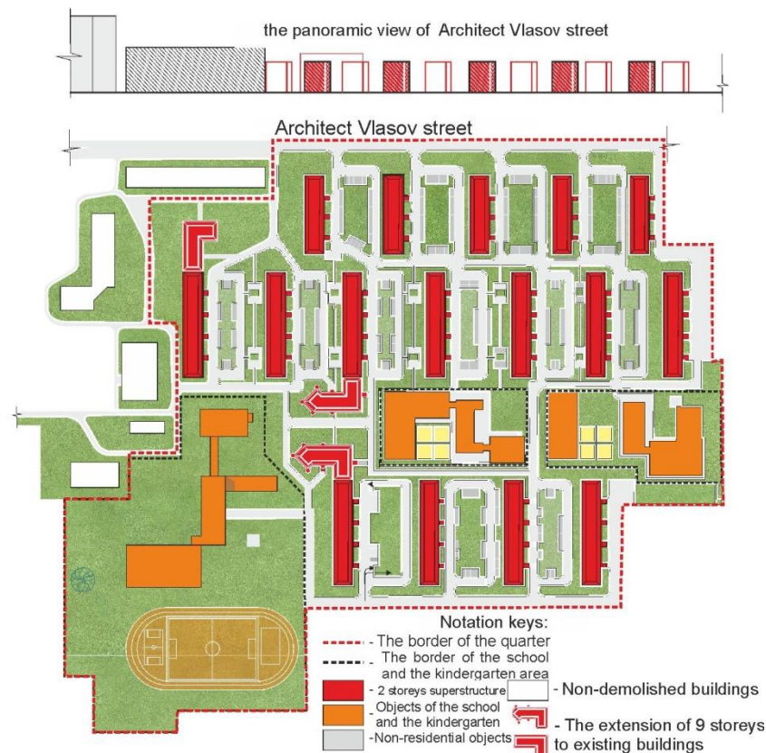
Figure 2. The renovation of the quarter without demolition of the residential buildings, without resettlement of the residents: a - the pre-project proposal; b - the fragment of the transformation of the landscape components of the development with the construction of the two-storey superstructures.
