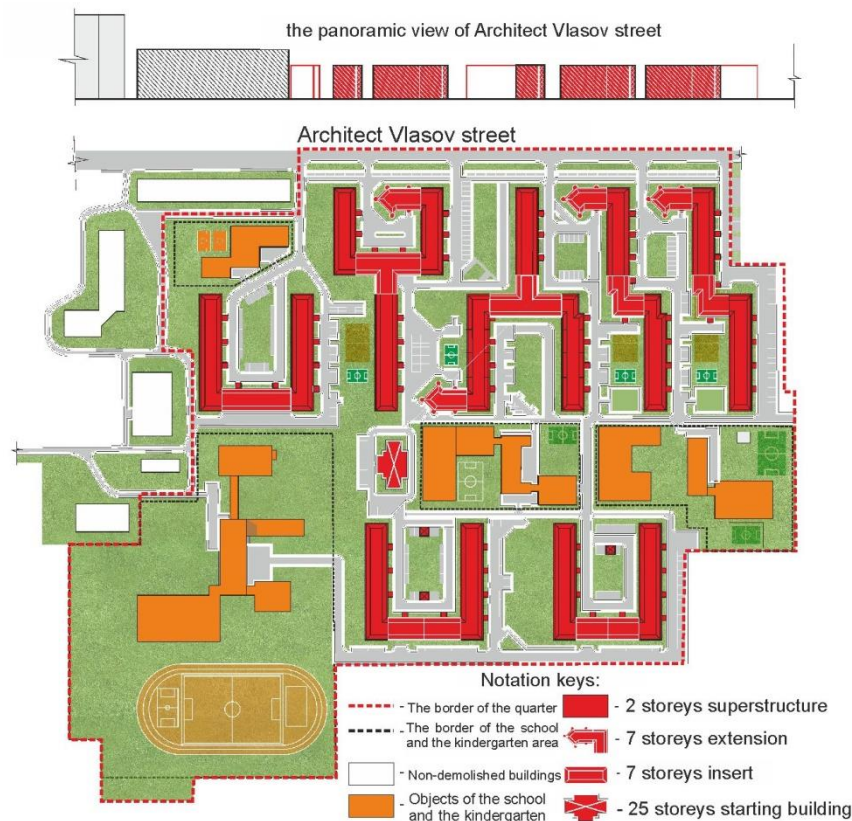
Figure 3. The renovation of the quarter without demolition of the residential buildings with resettlement of the residents: a - the pre-project proposal; b - the fragment of the transformation of the landscape components of the development with the construction of the two-storey superstructures, and the extensions, inserts.
