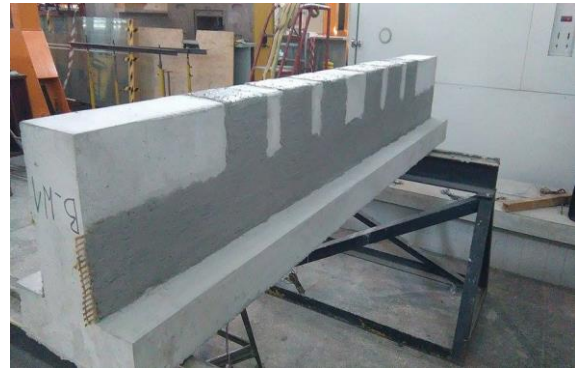
Figure 4. Anchorage after applying the outer layer of mortar
