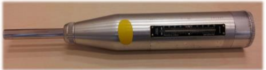
Figure 2. Rebound Schmidt hammer (type N) [2]
