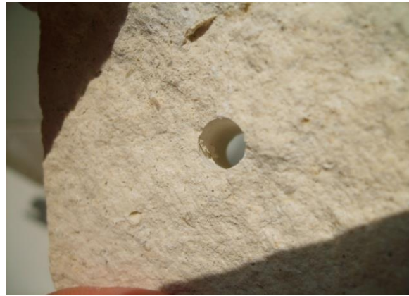
Figure 3. Flaking of the hole surface at the uniaxial compression of a limestone sample
