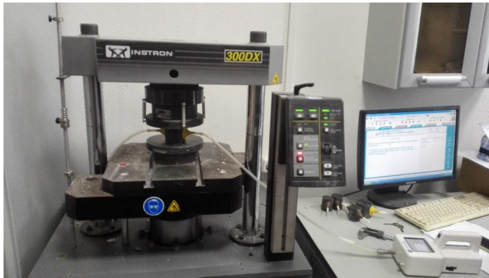
Figure 4. Experimental bench for laboratory investigations of the emission of submicron particles under different loading regimes
