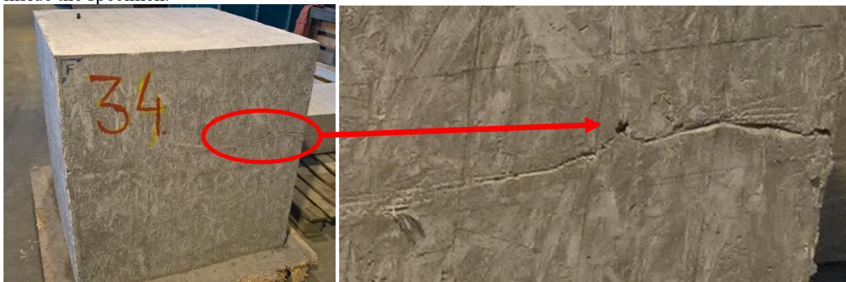
Figure 5. Picture of probe no. 34 and a zoom to longitudinal crack on it
