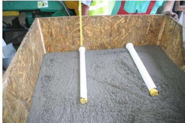
Figure 7. Additional insertions in concrete mix
