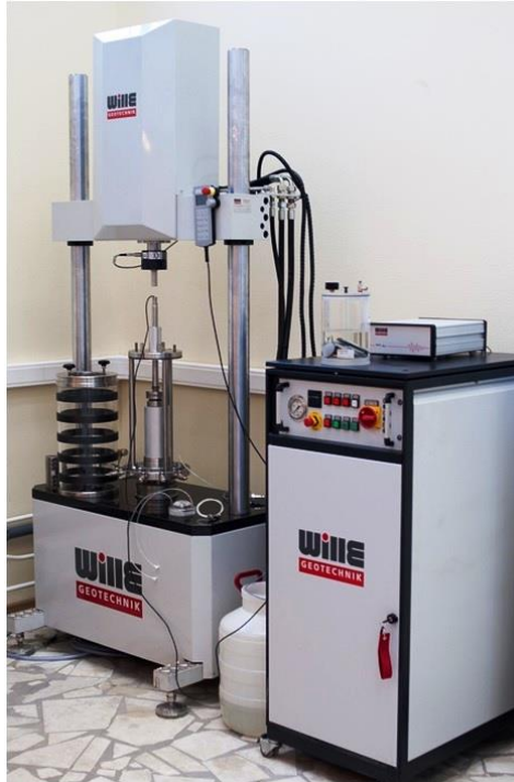
Figure 1. Equipment for triaxial testing of soils
