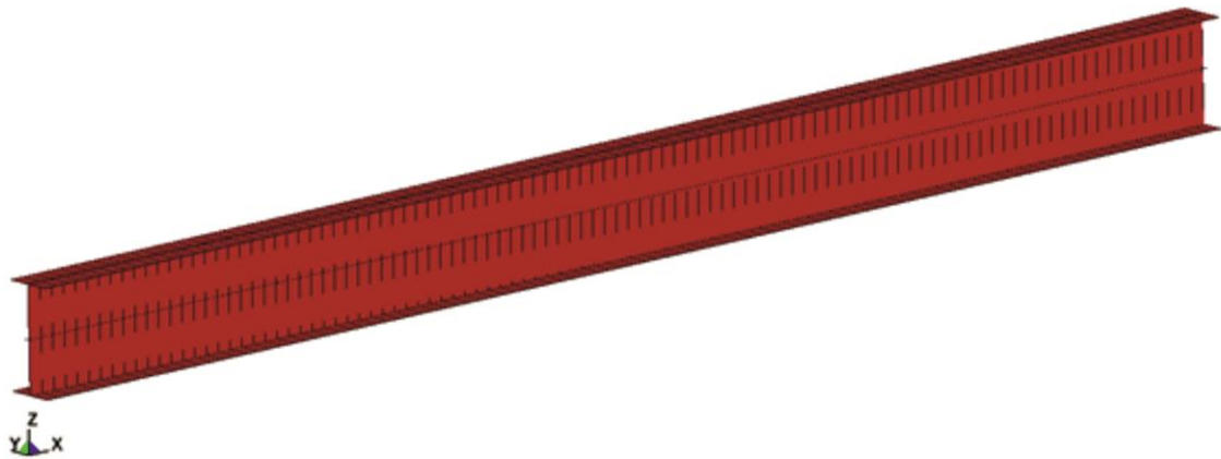
Figure 2. Hinge beam modeled with rod finite elements
