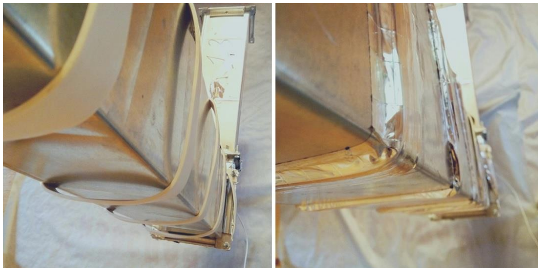
Figure 3. Photo of the experimental model. Left: resistance heating cable ENGL-1, right: cable fixation with self-adhesive aluminum reinforced tape
