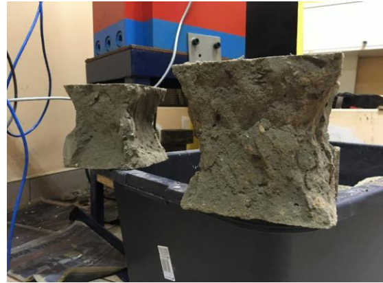
Figure 7. Example of samples destroyed (tested) one week after preparation
