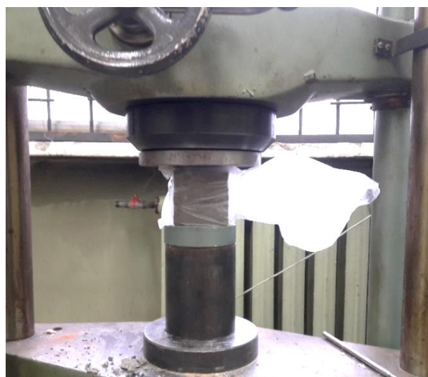
Figure 3. Testing a cube of cement for compression
