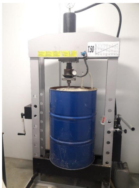
Figure 2. The general view of the tray test of the pile model
