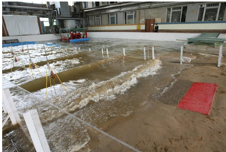
Figure 2. A large shallow pool of the ONIL Marine Oil and Gas Field Hydraulic Structures laboratory of the Moscow State University of Civil Engineering
