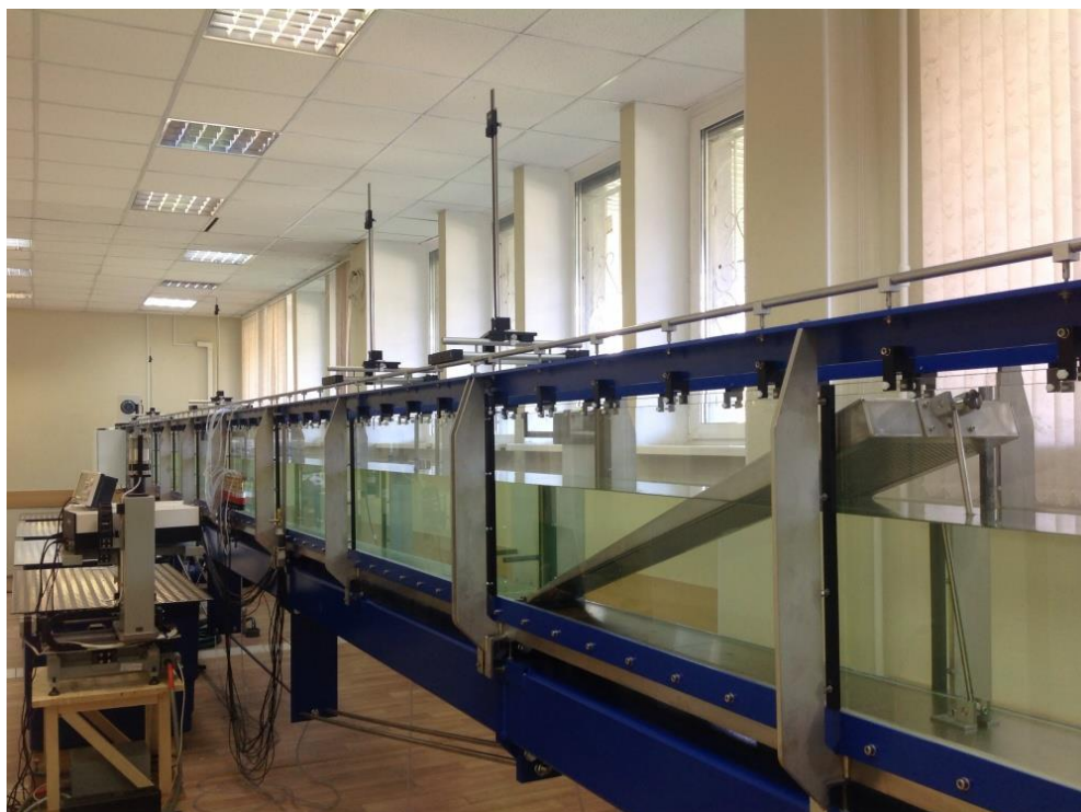
Figure 4. Hydraulic tray with variable gradient
