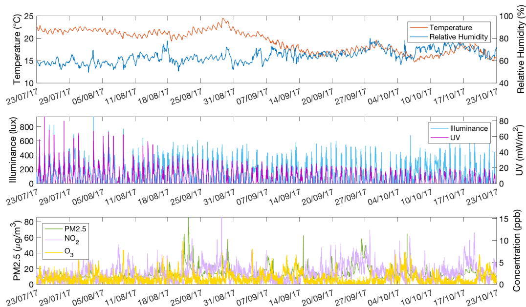
Figure 1. Environmental data registered for temperature, relative humidity, illuminance, ultraviolet radiation, particulate matter (PM 2.5 ), NO 2 and O 3 concentration.
