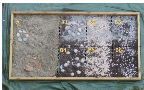
Figure 1. Mockup prepared in order to simulate an excavation site characterized by different texture and colours. A) six pebbles were placed on an almost uniform soil layer. A peat layer was partially covered by: B1) sand and a circle of 8 pebbles, B2) sand and a large quantity of gravel, B3) sand and a small quantity of gravel, B4) randomly-placed pebbles, B5) a large quantity of gravel, B6) a small quantity of gravel.
