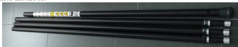
Figure 5. Monopod for shooting of tall sculptures with four section structure.
