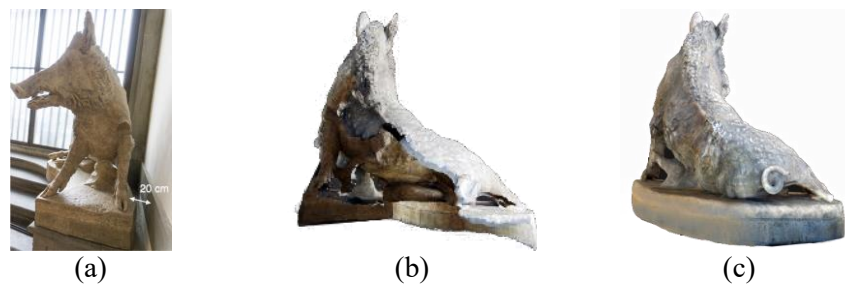
Figure 4. Sculptures close to the walls: a) example of sculpture having only 20 cm between the sculpted surface and the wall; b) model obtained with a 24mm lens, where a huge lacking part is present; c) model obtained with the 12 mm lens and the ring illuminator, completed in all areas close to the wall.
