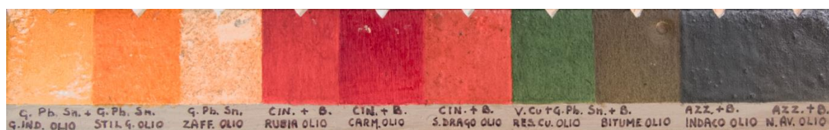
Fig. 1 A set of samples of pictorial layers. The triangle on the top of each swatch has been detached to be analysed under the standard optical microscope, SEM, and with the novel multispectral microscope.
