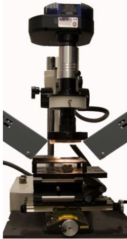
Fig. 4a The acquisition set-up. The microscope is coupled with a multispectral CCD camera
