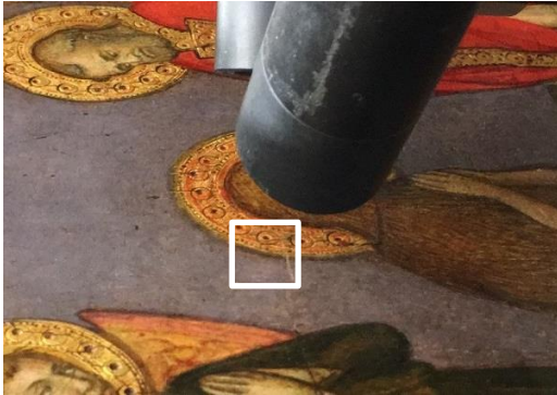
Figure 3. THz antennas analysing original pictorial sample. The box corresponds to the THz imaging area.
