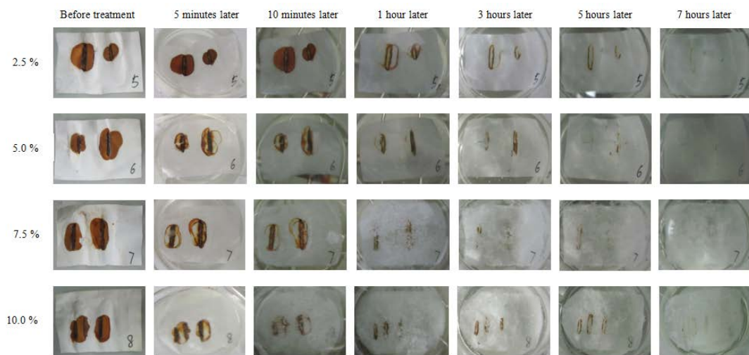
Fig. 5 The process of samples treated with different concentration TDO solutions( from up to down 2.5%, 5.0%, 7.5%, 10.0%) in 7 hours (from left to right: before treatment, 5 minutes later, 10 minutes later, 1 hour later, 3 hours later, 5 hours later and 7 hour later)
