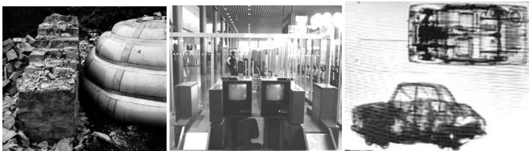
Figure 3. Left: Explosion-protection chamber based on damping of shock waves in water with gas bubbles, middle: X-ray complex at Sheremetyevo Airport, right: X-ray inspection of a car.
