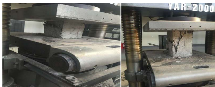
Figure 1. cube compressive strength and axial compressive strength test
