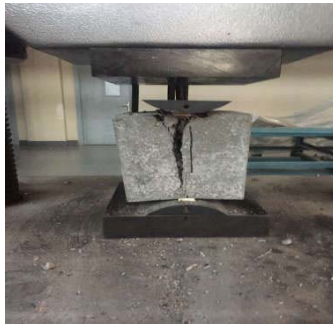
(a) Splitting failure
