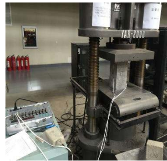
(b) Elastic modulus test
